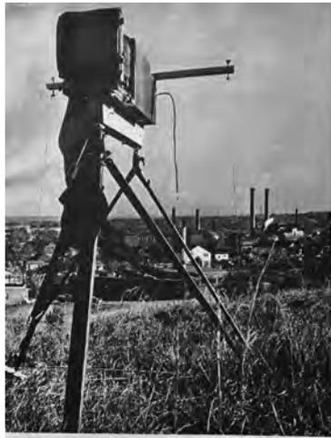
Feininger's home-built telecamera with 40" lens, above, set up on its free-legged "tripod" for a shot of New York City's skyline looking west-northwest. Groundglass on the front of the camera and anchored to the ground with pop wires is a wide-base to prevent vibrations of the lens board. Below, telephoto shot made on 8x8 film with 40" lens and camera setup above.
